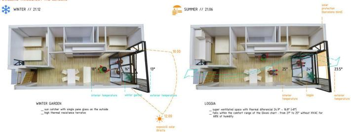
WINTER day: energy accumulation and radiation to the interior night: energy accumulation, radiation and max insulation
